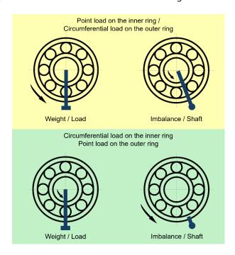
The following tables serve as a guide for selecting suitable fits between shaft and housing – depending on the load and direction of rotation in each case.
